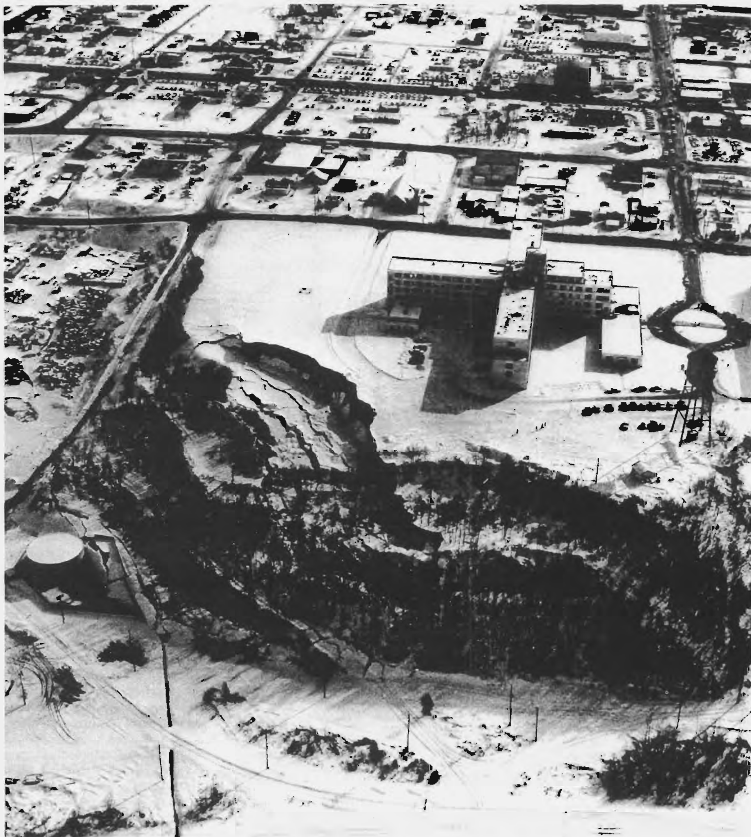
32.—Air view (looking south) of Native Hospital slide showing graben and pressure ridge. The scar of an older landslide is transected by the slide of March 27, 1964. Photograph by U.S. Army.
