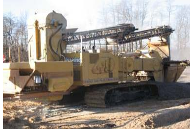
Trencher equipped with 25' bar, 2' wide cutter
