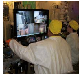
Operators at the controls for remote scabbling equipment
