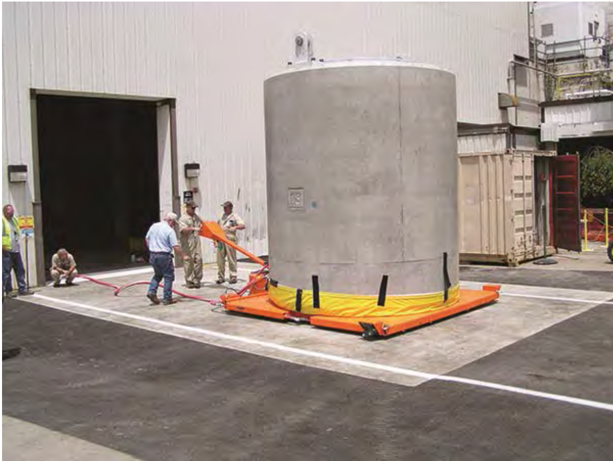
1. West Valley Nuclear utilizes a steel pallet with power drive to safely transport 87-ton casks of nuclear waste. Courtesy: AeroGo Inc.
