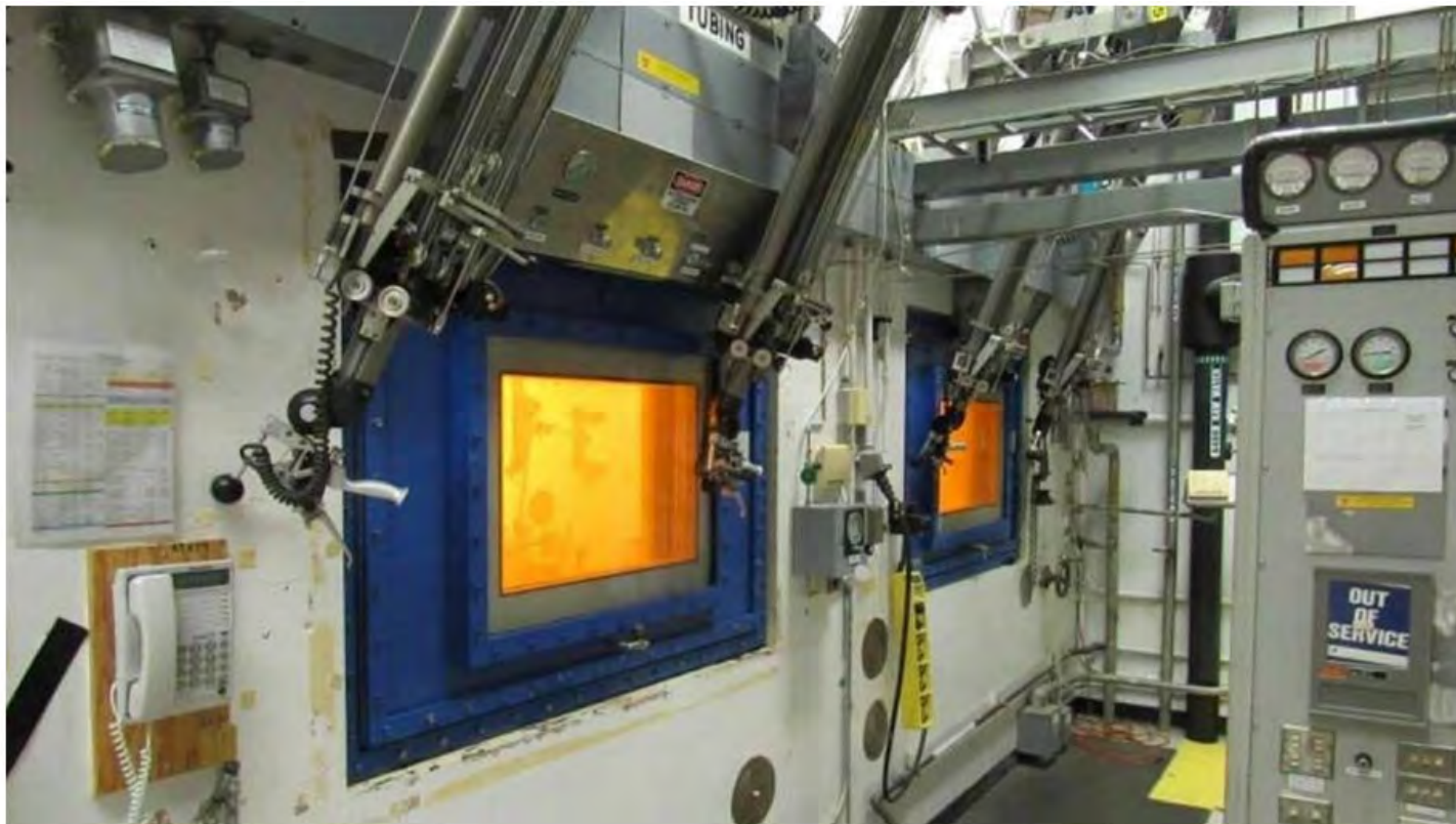
Hot cells at Hanford's Waste Encapsulation and Storage Facility will be used to prepare capsules of radioactive strontium and cesium for dry storage. DEPARTMENT OF ENERGY
